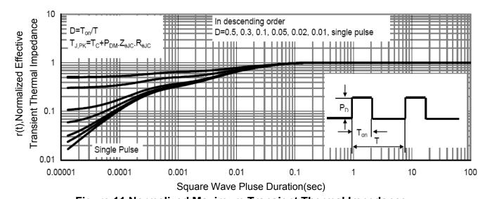
Figure 11 Normalized Maximum Transient Thermal Impedance
