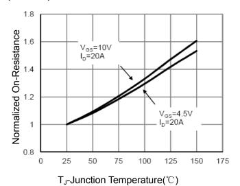
Figure 4 Rdson-Junction Temperature
