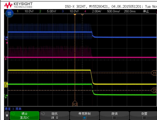
CH1: VIN CH2:VOUT CH3:SW CH4:IL Vin=5V Vout=5V Shut Down waveform through VIN, Iout =0A
