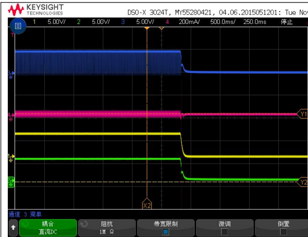
CH1: VIN CH2:VOUT CH3:SW CH4:IL Vin=5V Vout=5V Shut Down waveform through VIN, Iout =0A
