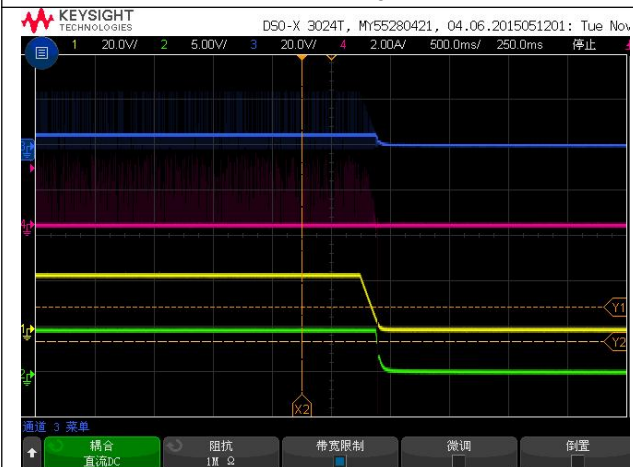
CH1: VIN CH2:VOUT CH3:SW CH4:IL Vin=12V Vout=5V Shut Down waveform through VIN, Iout =0A
