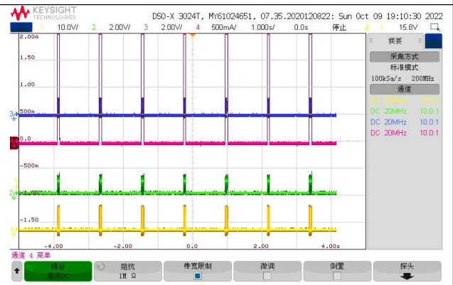
Fig.29 Load Transient IOUT=0-2A I-ramp=0.5A/us
