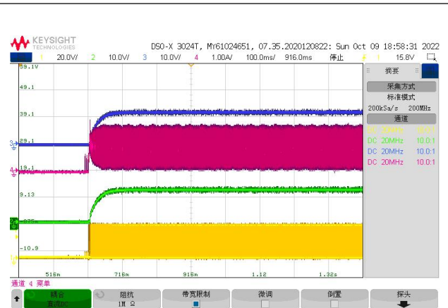
Fig.9 VIN Start up waveform, Iout =1A
