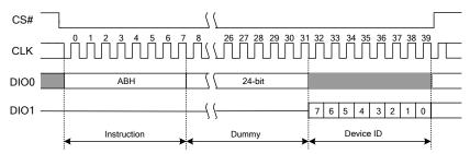
Figure 7.13 Release Power-down / Device ID Instruction Sequence Diagram
