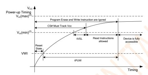
Figure 8.1 Power-up Timing
