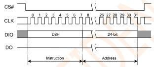
Figure 7.9 Block Erase Instruction Sequence Diagram
