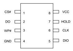
Figure 3.1 8-pin SOP (150/208mil)/ PDIP (300mil)
