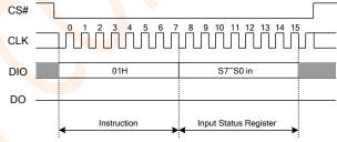
Figure 7.4 Write Status Register Instruction Sequence Diagram
