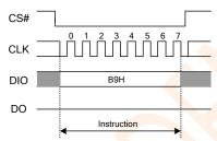
Figure 7.11 Deep Power-down Instruction Sequence Diagram
