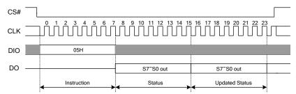
Figure 7.3 Read Status Register Instruction Sequence Diagram
