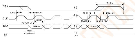
Figure 8.4 Input Timing
