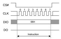
Figure 7.1 Write Enable Instruction Sequence Diagram
