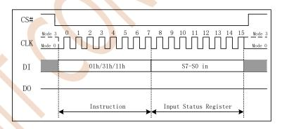
Figure 7.5 Write Status Register Instruction (SPI Mode)
