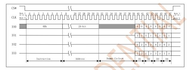
Figure 7.16 Fast Read Quad Output Instruction
