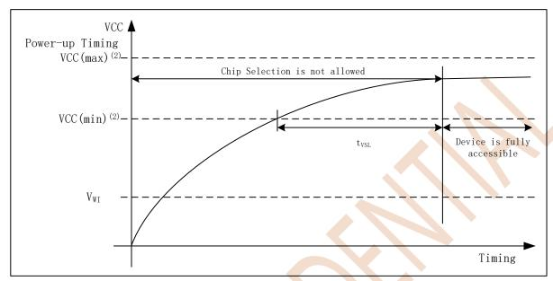
Figure 8.1 Power-up Timing
