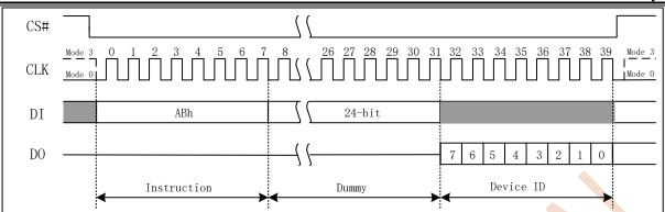
Figure 7.25 Release Power-down / Device ID
