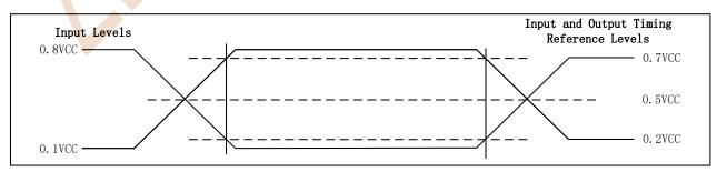
Figure 8.3 AC Measurement I/O Waveform
