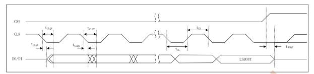
Figure 8.4 Serial Output Timing
