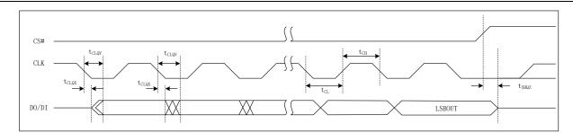
Figure 8.4 Serial Output Timing
