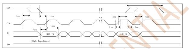
Figure 8.5 Input Timing
