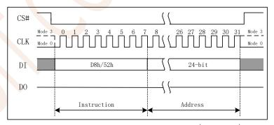
Figure 7.9a Block Erase Instruction (SPI Mode)
