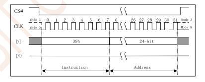
Figure 7.32a Individual Block/Sector Unlock Instruction(SPI Mode)
