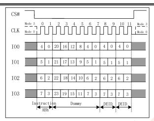
Figure 7.24b Release Power-down / Device ID(QPI Mode)
