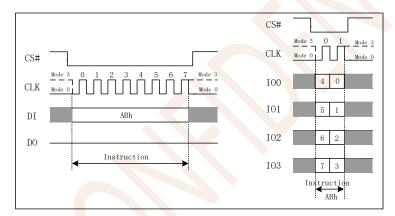
Figure 7.23 Release Power-down Instruction (SPI and QPI Mode)
