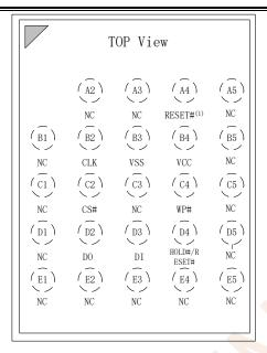
Figure 3.4 24-BALL TFBGA (5x5 ball array)
