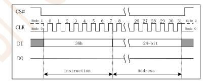
Figure 7.31a Individual Block/Sector Lock Instruction(SPI Mode)
