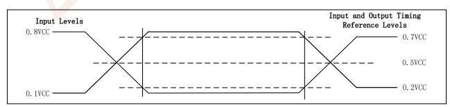
Figure 8.3 AC Measurement I/O Waveform
