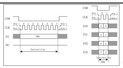
Figure 7.35 Global Block Lock Instruction (SPI or QPI Mode)
