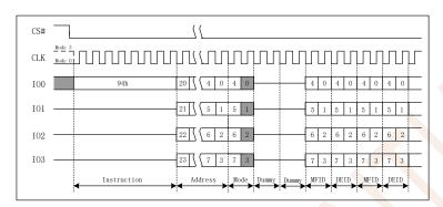
Figure 7.37 Read Manufacturer/Device ID Quad I/O Instruction
