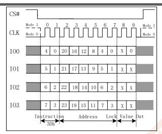
Figure 7.33b Read Block Lock Instruction (QPI Mode)
