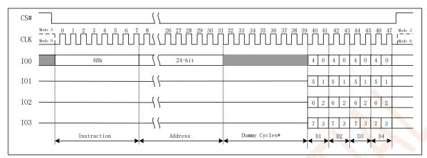
Figure 7.16 Fast Read Quad Output Instruction
