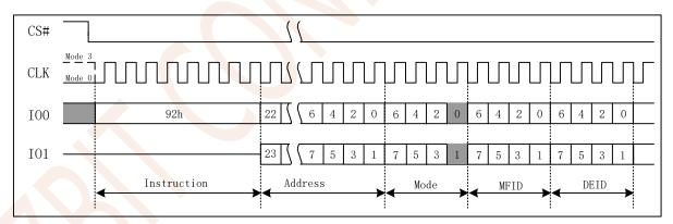
Figure 7.36 Read Manufacturer/Device ID Dual I/O Instruction
