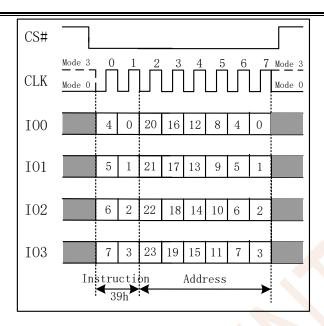
Figure 7.32b Individual Block/Sector Unlock Instruction (QPI Mode)
