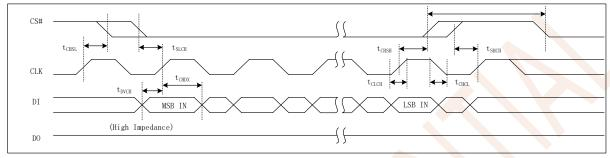
Figure 8.5 Input Timing
