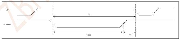
Figure 8.8 Hardware Reset Timing
