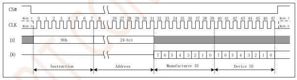
Figure 7.25a Read Manufacturer/Device ID(SPI Mode)
