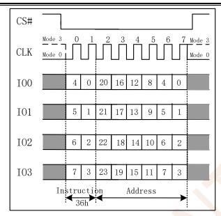
Figure 7.31b Individual Block/Sector Lock Instruction (QPI Mode)
