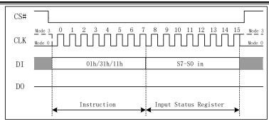
Figure 7.5a Write Status Register Instruction (SPI Mode)
