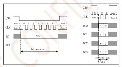
Figure 7.34 Global Block Lock Instruction (SPI or QPI Mode)
