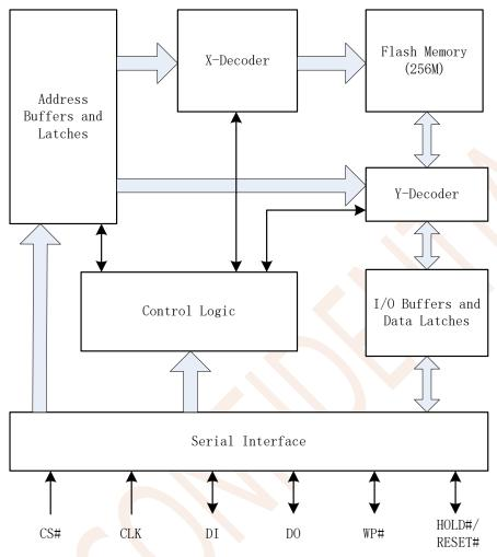
Figure 2.1 Block Diagram
