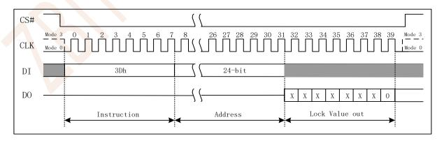
Figure 7.33a Read Block Lock Instruction(SPI Mode)
