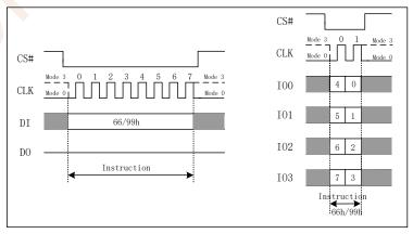
Figure 7.21 Software Reset Instruction (SPI and QPI Mode)
