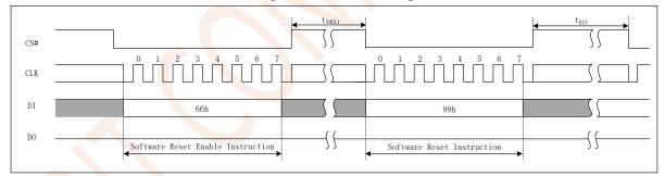
Figure 8.7 Software Reset Input Timing
