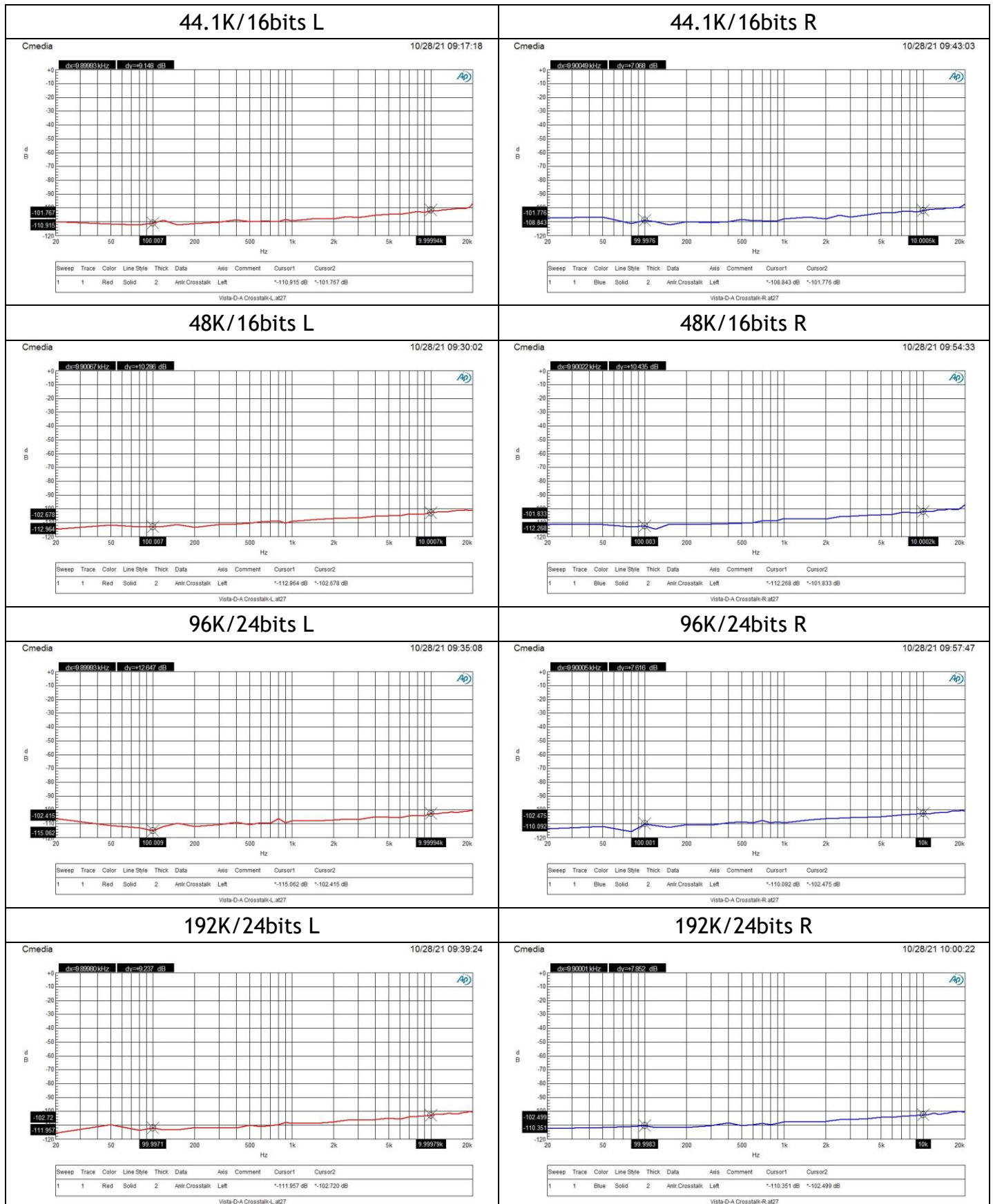
Figure 7 : DAC 10K \Omega loading, Cross-talk
