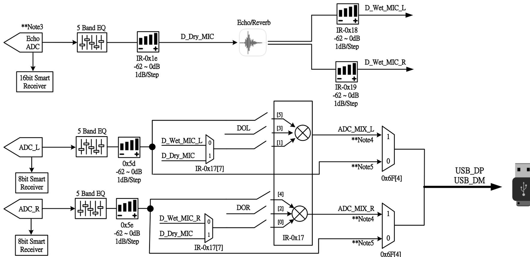
\*\*Note3: The Echo ADC path only support 48K/16 bit sampling rate
