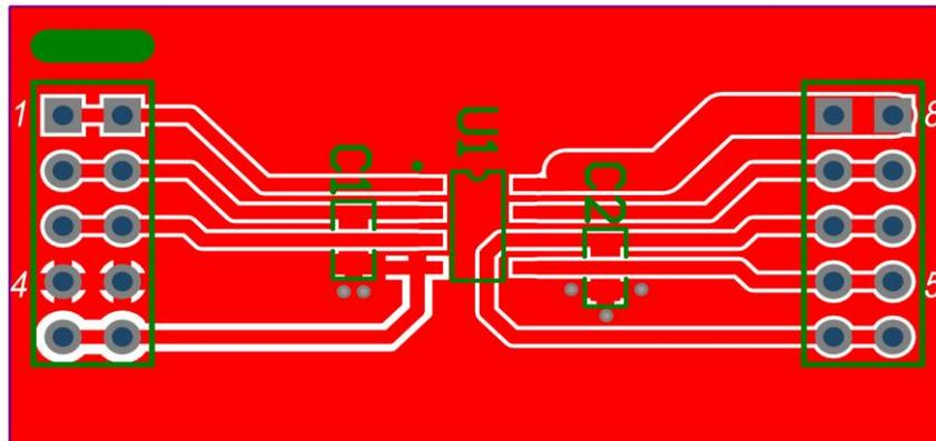
Figure 27. ZJR1000 Evaluation Board Layout (Top Layer)
