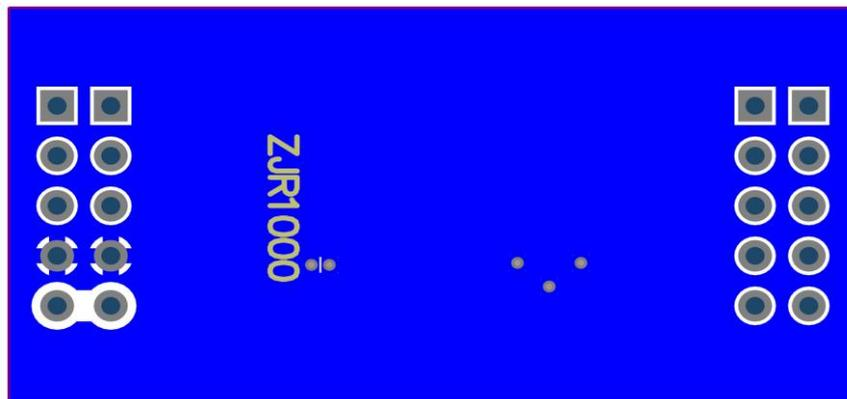
Figure 28. ZJR1000 Evaluation Board Layout (Bottom Layer)
