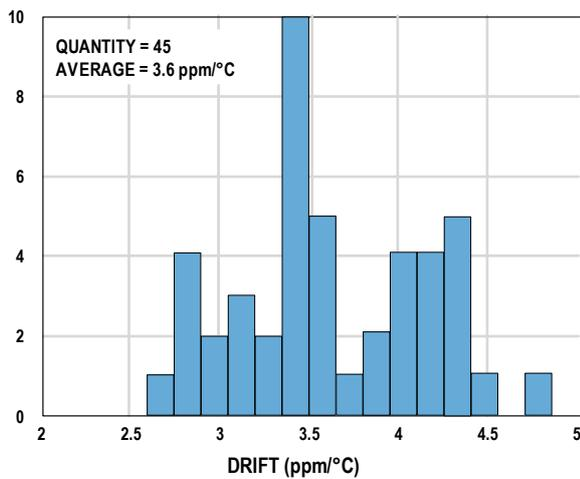
Figure 18. ZJR1000-9 Temperature Coefficient Distribution (MSOP-8 package)
