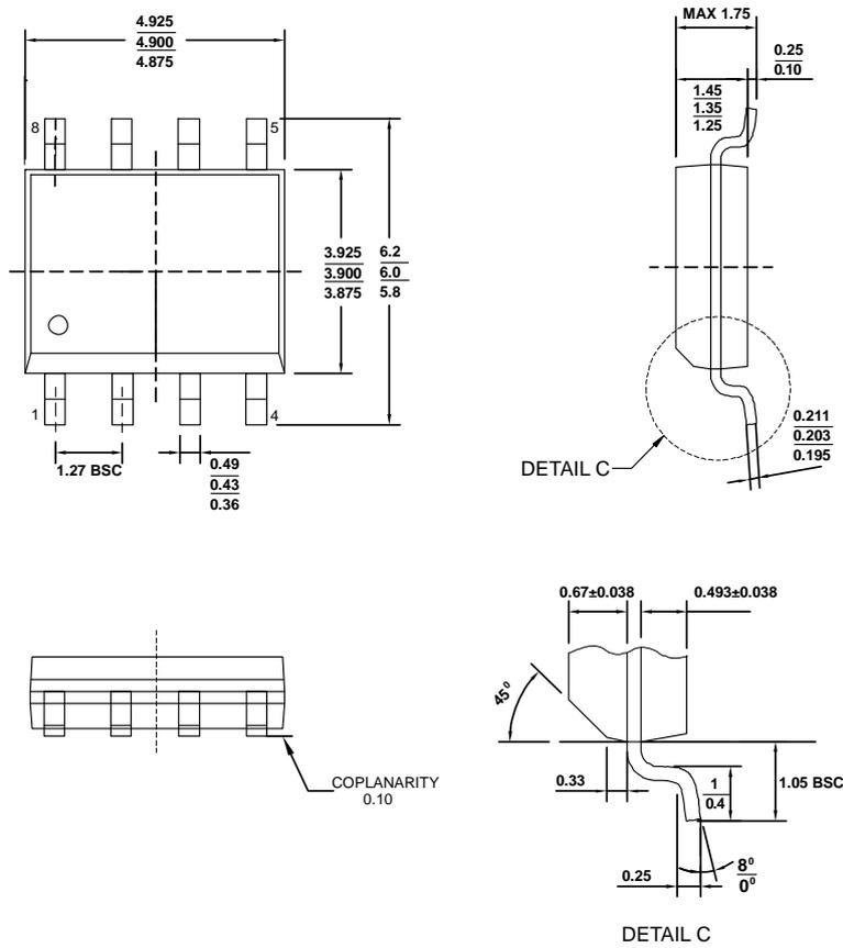
Figure 29. 8-Lead SOIC Package Dimensions shown in millimeters
