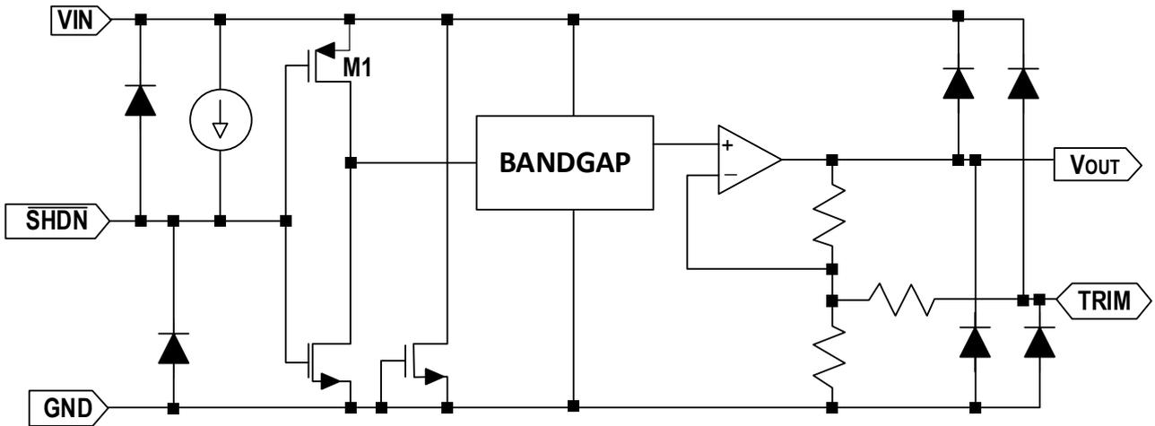
Figure 20. Simplified Schematic of ZJR1000
